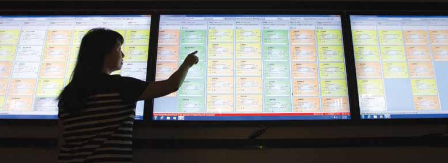
*At Littlestar Plastics, a moldmaker based in Rockford, IL, an employee enters shop-floor information using the big-screen electronic scheduling board developed by Henning Industrial Software for use with its Visual EstiTrack ERP program.*
